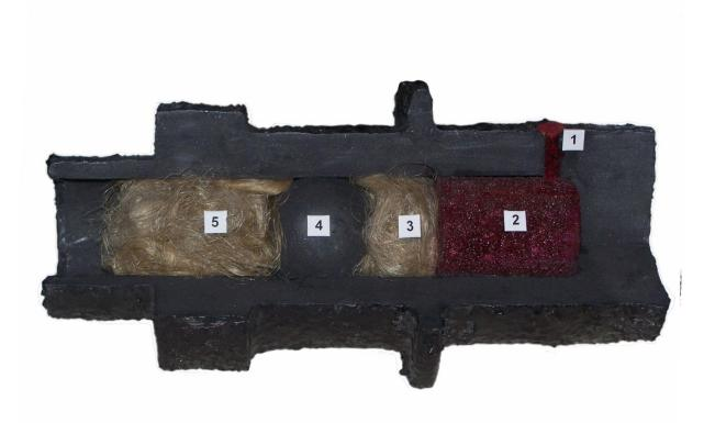
Fig. 1: Diagram of a muzzle-loader. (1) Priming charge, (2) Main propellant charge, (3) and (5) Wadding, (4) Projectile (from http://upload.wikimedia.org/wikipedia/commons/9/91/CMM\_-\_Przekr%C3%B3j\_mo%C5%BAdzierza.JPG)
